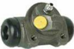
5. 673 558 links/left System: Bendix Ø 19,05 mm + 4x4
